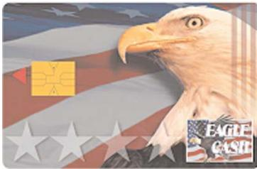
Accounting Service, the Army and Air Force Exchange Service (AAFES), and the Army. The card is the size of a standard credit card and has an embedded microprocessor chip that holds information in electronic form.
